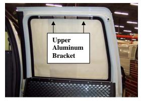
Hold window guard with pre-assembled hinge and upper bracket onto window frame. Make sure guard is centered on window. Attach hinge to lower door panel with #10 x  $\frac{1}{2}$ " stainless sheet metal screws. Mark upper aluminum bracket location on window frame and remove from window guard. Attach upper aluminum bracket onto window frame with #10 x  $\frac{1}{2}$ " flat head sheet metal screws.
